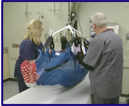
Figure 4. Powered ceiling or overhead lift used to reposition a patient in bed
