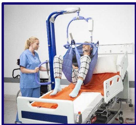
Figure 5.13 Sufficient Vertical/Lift Clearance from a Surface.
