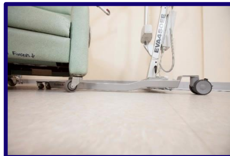
Figure 5.12 Low-Based Floor Lift with Sufficient Clearance Under a Chair.
