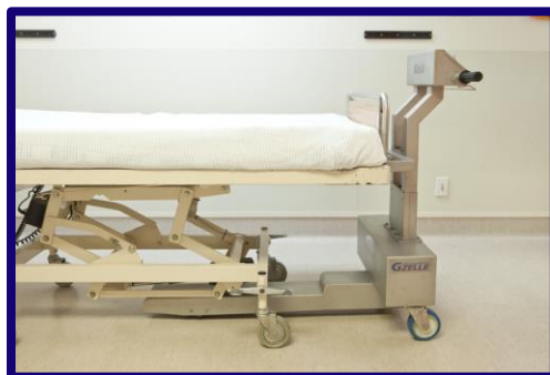
Figure 5.36 Example of a Battery Powered Transport Assist for Non-Motorized Beds.
