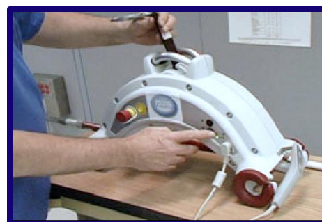
Figure 5.4 Example of a Portable Overhead Lift Motor.
