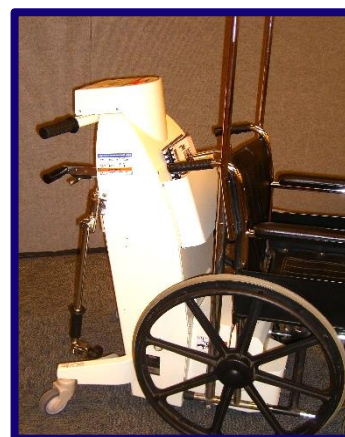
Figure 5.37 Example of a Battery Powered Transport Assist for Wheelchairs.
