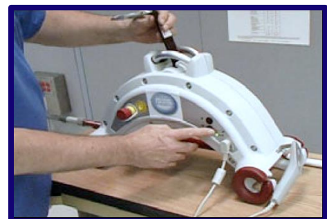
Figure 5.4 Example of a Portable Overhead Lift Motor.
